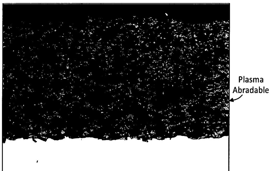
Microstructure of a Crack-Free Abradable Coating Applied on a Superalloy Substrate
