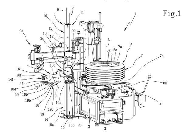
[0001] This invention relates to a device for lifting a bottom side wall of a tyre in a tyre removing machine (in particular in a tyre removing machine where the tyre to be removed is positioned with its axis vertical).
