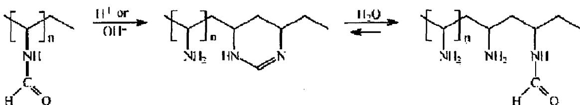
45 **[0036]** Wherein amide moieties in the copolymer react via intramolecular reaction to produce the amidine rings. The presence of such rings may be determined by <sup>13</sup>CNMR as shown in Figure 3.
