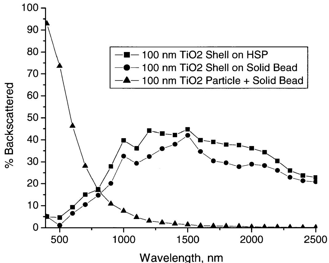
Comparative Example 2: Theoretical Calculations of Backscattering of Various Bead Types - TiO<sub>2</sub> particle = 160nm
