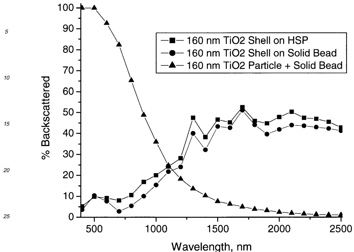
Comparative Example 3: Theoretical Calculations of Backscattering of Various Bead Types - TiO<sub>2</sub> particle = 200nm
