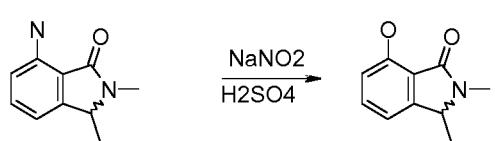
50 [0084] 7-amino-2,3-dimethyl-2,3-dihydro-isoindol-1-one (11.45 g) is suspended in a mixture of ice (27 g) and  $\text{H}_2\text{SO}_4$  conc. (9.70 mL) and cooled to -10°C. Aqueous sodium nitrite solution (2.5 molar, 31.18 mL) is added dropwise, so that the temperature does not rise above 0°C and the solution is stirred for 15 min at this temperature. Then  $\text{H}_2\text{O}$  (135 mL)
