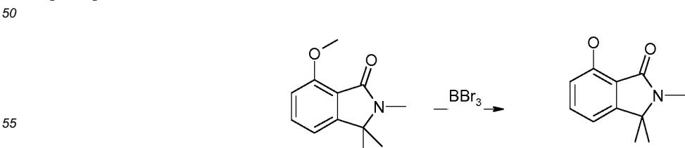
[0097] 7-methoxy-2,3,3-trimethyl-2,3-dihydro-isoindol-1-one (0.18 g) is dissolved in CH<sub>2</sub>Cl<sub>2</sub> (4.5 mL) and cooled to
