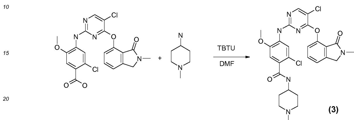
25     **[0114]** 2-chloro-4-[5-chloro-4-(2-methyl-3-oxo-2,3-dihydro-1*H*-isoindol-4-yloxy)-pyrimidin-2-ylamino]-5-methoxybenzoic acid (65 mg), TBTU (60 mg) and DIPEA (0.1 mL) are suspended in DMF (0.50 mL) and stirred for 5 min. 1-methylpiperidin-4-amine (18 mg) is added and the reaction mixture is stirred for a further 20 min. The reaction mixture is purified by HPLC without working up. ( $\text{IC}_{50} = 1 \text{ nmol}$ ).
