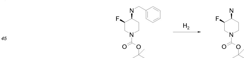
[0106] Tert-butyl (3R,4S)-4-benzylamino-3-fluoro-piperidine-1-carboxylate (2.13 g) is suspended in THF and mixed with a spatula tip of Pd(OH)<sub>2</sub> and hydrogenated under H<sub>2</sub> pressure (7 bar). For working up the catalyst is filtered off and the solvent is eliminated in vacuo and the residue is used in the next step without any further purification.
