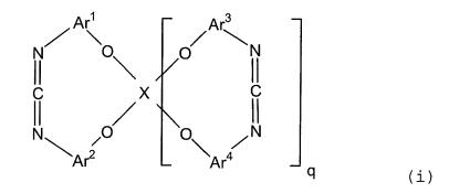
(in the above formula, X is any one of divalent groups represented by the following formulas (i-1) to (i-3) or a tetravalent group represented by the following formula (i-4), when X is divalent, q is 0 and when X is tetravalent, q is 1, and  $Ar^{1}$  to  $Ar^{4}$  are each independently an aromatic group and may be substituted by an alkyl group having 1 to 6 carbon atoms or phenyl group)
