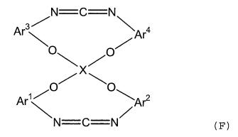
**[0021]** In the above formula,  $Ar^1$  to  $Ar^4$  and X are as defined in the formula (i).  $Ar^1$  to  $Ar^4$  are each preferably an ophenylene group which may be substituted. The substituent is preferably an alkyl group having 1 to 6 carbon atoms or phenyl group. X is a tetravalent group.
