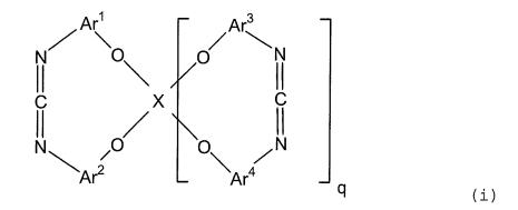
**[0010]** In the above formula, Ar<sup>1</sup> to Ar<sup>4</sup> are each independently an aromatic group. The aromatic group may be substituted by an alkyl group having 1 to 6 carbon atoms or phenyl group. Examples of the aromatic group include aromatic groups having 5 to 15 carbon atoms such as phenylene group and naphthalenediyl group.
