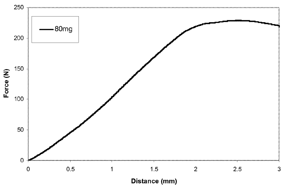
Example 20 Indentation Test of Example 16.2 tablet
