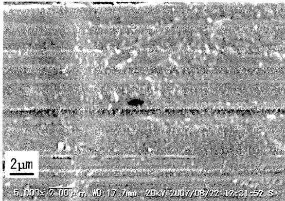
Drawing temperature 330°C Drawing rate 0.8m/min
