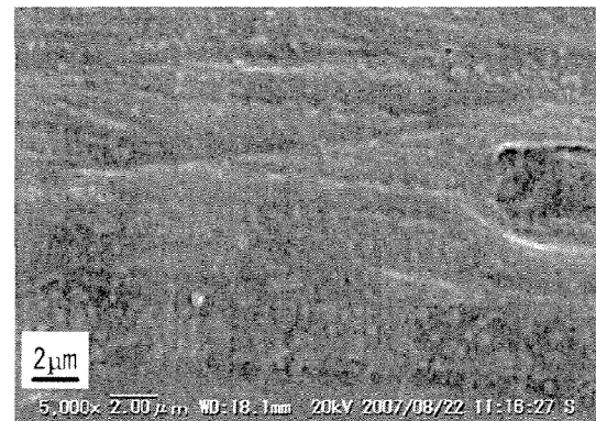
Drawing temperature 400°C Drawing rate 8.4m/min
