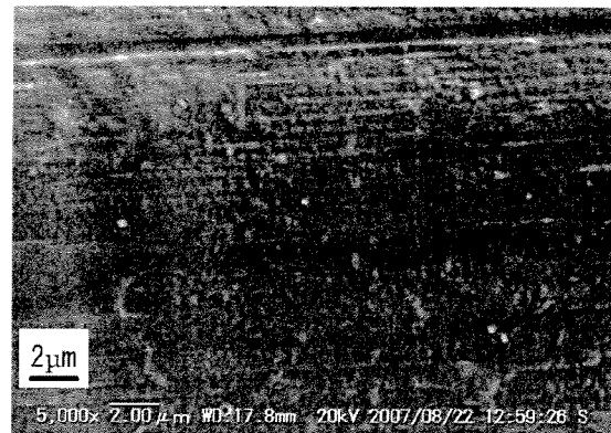
Drawing temperature 330°C Drawing rate 2.8m/min
