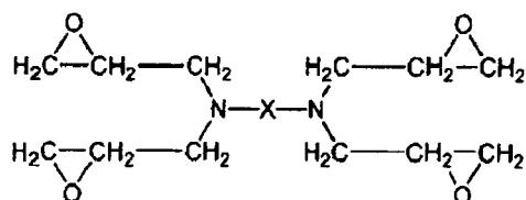
wherein X is alkyl having 1 to 30 carbon atoms or an aryl group, in which X optionally contains oxygen, nitrogen or the like.
