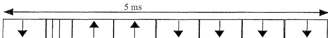
Configuration of uplink and downlink time slots in an unsymmetrical service
