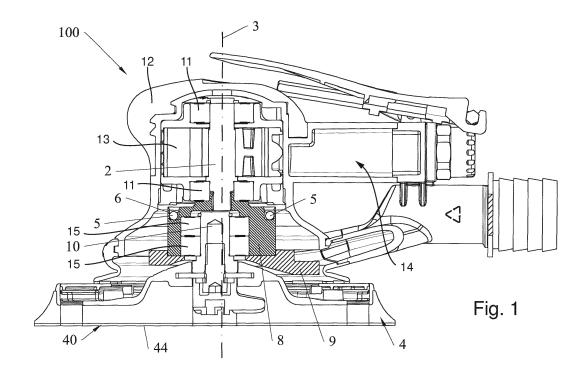
**[0001]** The present invention refers to a machine tool performing a rotary orbital, a random orbital or an orbital movement and provided with a balancing system, in order to minimize vibrations of the tool while functioning. In particular the invention refers to a machine tool comprising
