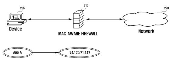
App A wants to write data to the socket for IP address 74.125.71.147
