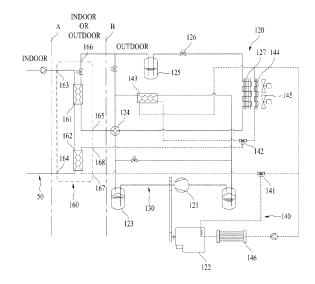
[0001] The present invention relates to a gas heat pump system which uses a gas engine, and more particularly to a gas heat pump system for driving a compressor to realize a refrigerating cycle by using a gas engine.
