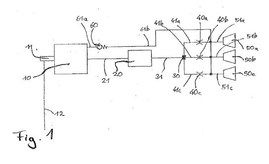
**[0001]** The invention relates to an aircraft oxygen emergency device comprising a chemical oxygen generator, an oxygen supply line including a first line section connecting said chemical oxygen generator with a flow regulator unit and a second line section connecting said flow regulator unit with at least one oxygen mask for supplying oxygen to mouth and/or nose of a person at a breathing pressure.
