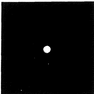
Nanobeam electron diffraction image Point A Beam diameter : About 5nm \phi
