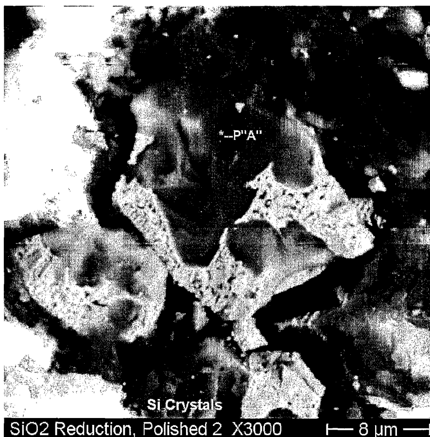
Fig. 16. Silicon crystal found in the pellet after reduction
