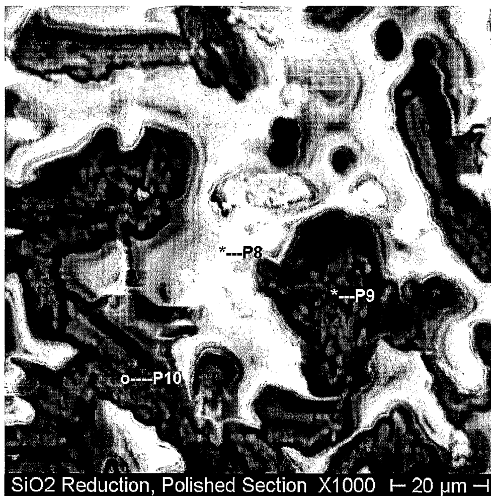
Fig. 10. Appearance of the structure of the SiO 2 pellet after reduction
