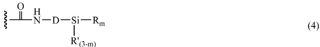
wherein D is straight or branched C<sub>1</sub>-C<sub>8</sub> alkylene group, each R independently is a hydrolysable group, each R' independently is a C<sub>1</sub>-C<sub>4</sub> alkyl group, and m is an integer of 1 to 3 are low volatile and serve to enhance the adhesion of resins to inorganic substrates.
