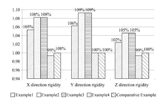
[0034] As can be seen from the above graph, according to the tire tread block structure of an exemplary embodiment
