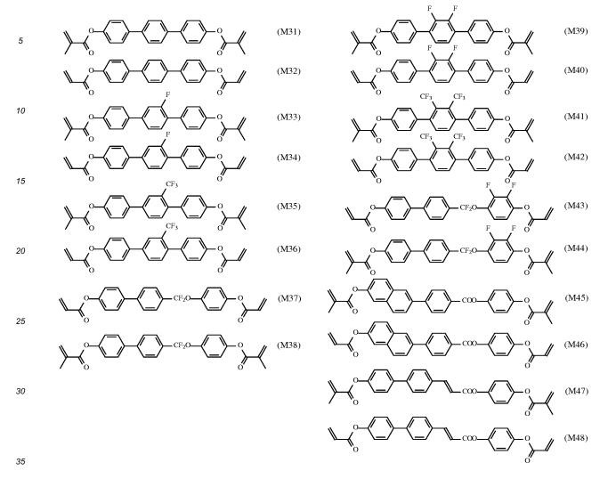
**[0066]** A hydrogen atom of the phenyl group or the naphthalene group represented in Formulae (M31) to (M48) may be replaced by -F, -Cl, -CF<sub>3</sub>, -CH<sub>3</sub>, or any one of the structures represented by Formulae (R-1) to (R-15).
