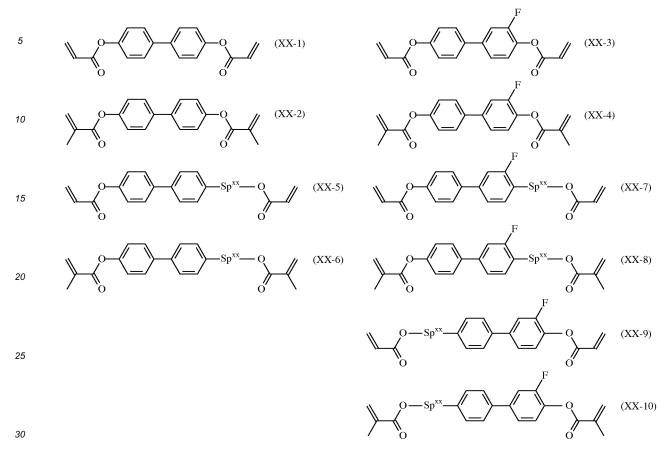
**[0064]** In Formulae (XX-1) to (XX-10),  $Sp^{xx}$  represents an alkylene group having 1 to 8 carbon atoms or  $-O-(CH_2)_s$ -(where s is an integer of 2 to 7 and the oxygen atom is bonded to the ring).
