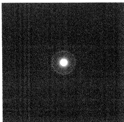
Selected-area electron diffraction image Point C Selected-area diameter: Approximately 600nm \phi Camera Constant L \cdot \lambda = 20.06 \text{ \AA} \cdot \text{mm}
