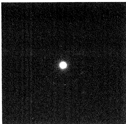
Nano-beam electron diffraction image Point A Beam diameter: Approximately 5nm \phi
