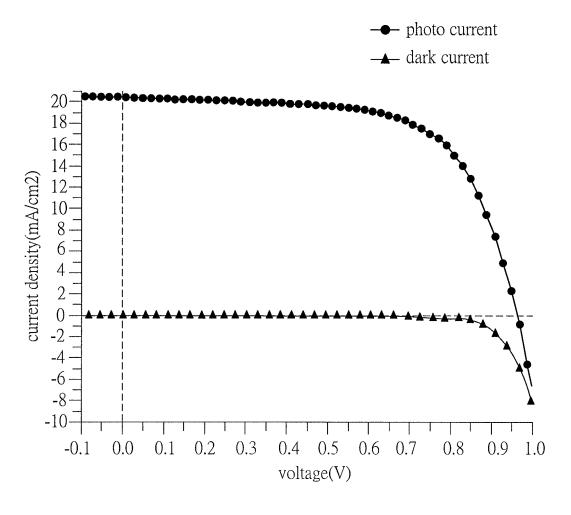
short-circuit current density =20.35mA/cm2 open-circuit voltage =0.96V fill factor =0.65 PCE =12.86%
