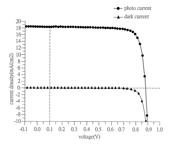
short-circuit current density =18.33mA/cm2 open-circuit voltage =0.88V fill factor =0.81 PCE =13.10%
