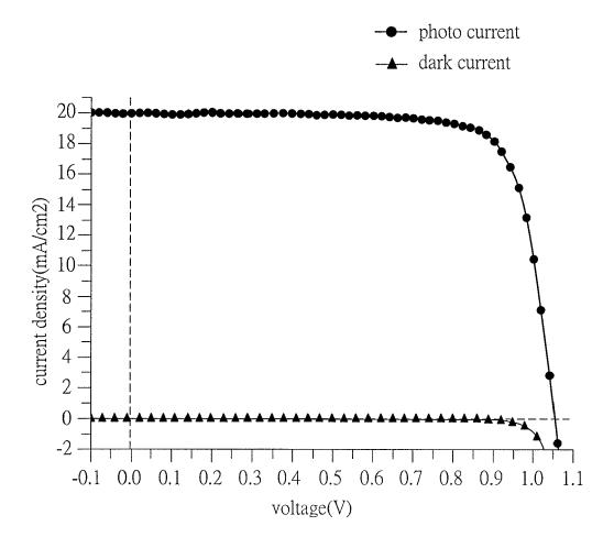
short-circuit current density =19.98mA/cm2 open-circuit voltage =1.05V fill factor =0.77 PCE =16.15%
