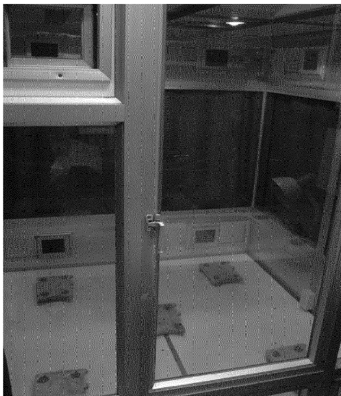
Figure 20. Space Spray for House Fly control in a Peet Grady Chamber
