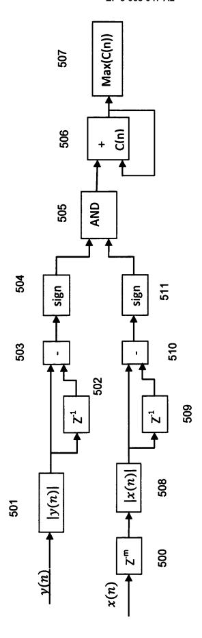
FIG. 5. Delay Estimation Block
