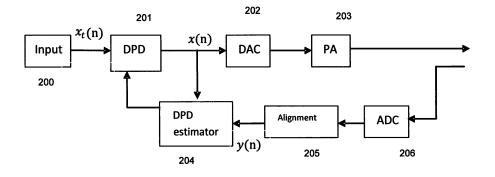
FIG. 2. Digital Predistortion Block Diagram
