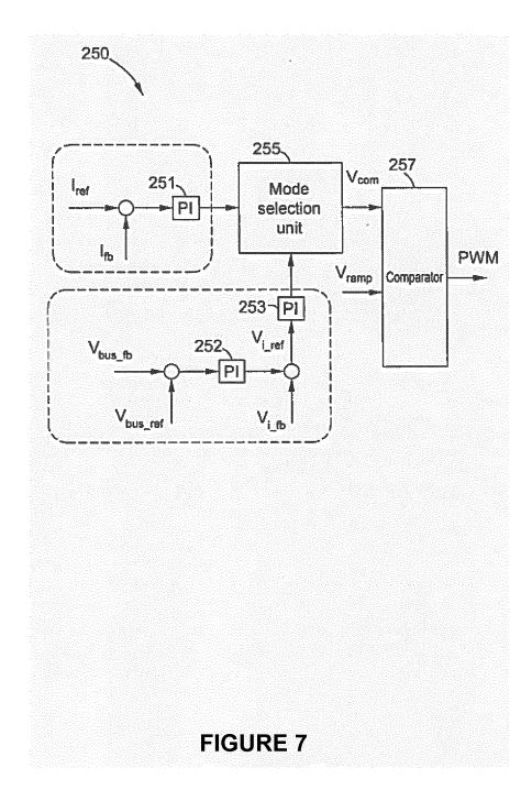
The operation includes a first energy storage system, a second energy storage system and a second DC-DC converter storage system for multi-source energy. The precharge mode, includes using the first energy storage system to charge the second energy storage system via the second DC-DC converter.
