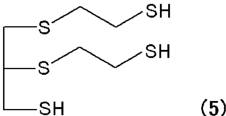
15 [0025] Step D: Hydrochloric acid which is a concentration of 25% to 36% is added to the solution containing the polythiol compound obtained in step C, the solution is washed at a temperature of 10°C to 50°C, and the polythiol compound is purified.
