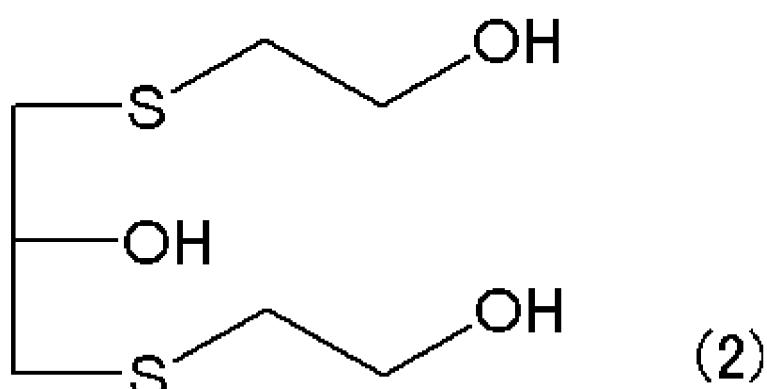
55 a step for reacting the polyalcohol compound represented by formula (2) thus obtained with thiourea in the presence of hydrogen chloride to obtain an isothiuronium salt;
