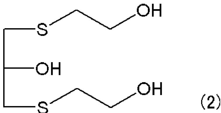
[a4] The method for producing a polythiol compound according to [a3], wherein the step for reacting 2-mercptoethanol with an epihalohydrin compound includes
