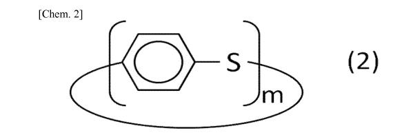
[0033] The PPS cyclic oligomer may be either a single compound in which the molecules are equal in the number of repetitions or a mixture of PPS cyclic oligomer compounds differing in the number of repetitions. However, a mixture of PPS cyclic oligomer compounds differing in the number of repetitions is preferred because this mixture tends to have a lower melting temperature than single compounds in each of which the molecules are equal in the number of repetitions.
