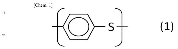
**[0025]** From the standpoint of heat resistance, the PPS preferably is a polymer which includes the repeating units represented by structural formula (1) in an amount of 70% by mole or larger, desirably 90% by mole or larger.
