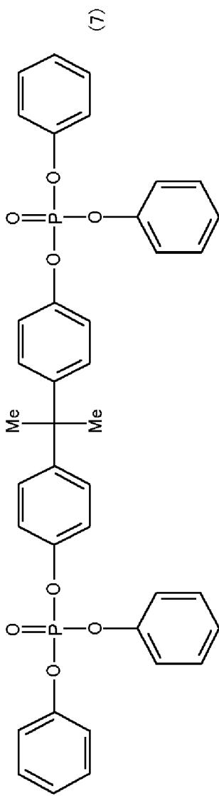
[0076] In the comparative example 1, a uniform prepreg could not be obtained, for the reason that the phosphorus-containing compound used was crystallized when the prepreg was manufactured, therefore, subsequent evaluations could not be made. In the comparative example 2, a uniform laminated plate could not be obtained, for the reason that a component which seems to be FP-600 is partially separated in pressure curing when the both sides copper-clad laminated plate was manufactured.
