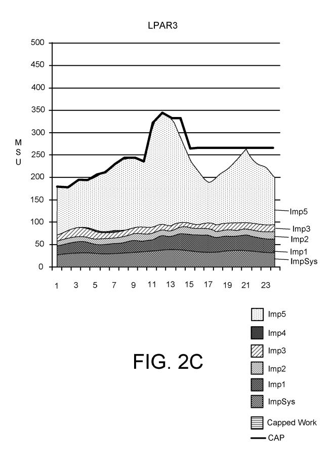
Querying a Workload Manager (WLM) component of the LPAR O/S to determine recent consumption of MSUs by importance level of work for each entity (e.g., LPAR or capacity group) in the managed group of system usage entities 310
