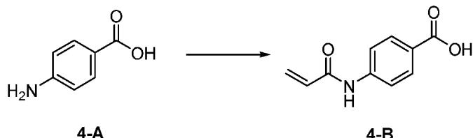
[0167] A solution of 4-aminobenzoic acid (1.40 g, 10 mmol) in DMF (10 mL) and pyridine (0.5 ml) was cooled to 0° C. To this solution was added acryloyl chloride (0.94 g, 10 mmol) and the resulting mixture was stirred for 3 hours at RT. The mixture was poured into 200 ml of water and the white solid obtained was filtered, washed with water and ether, dried to afford the title compound which was used in the next step without purification (1.8g) LCMS: m/z = 192.1 (M+H)<sup>+</sup>.
