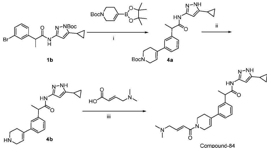
Step-i: Synthesis of tert-butyl 4-(3-((5-cyclopropyl-1H-pyrazol-3-yl)amino)-1-oxopropan-2-yl)phenyl)-3,6-dihydropyridine-1(2H)-carboxylate
