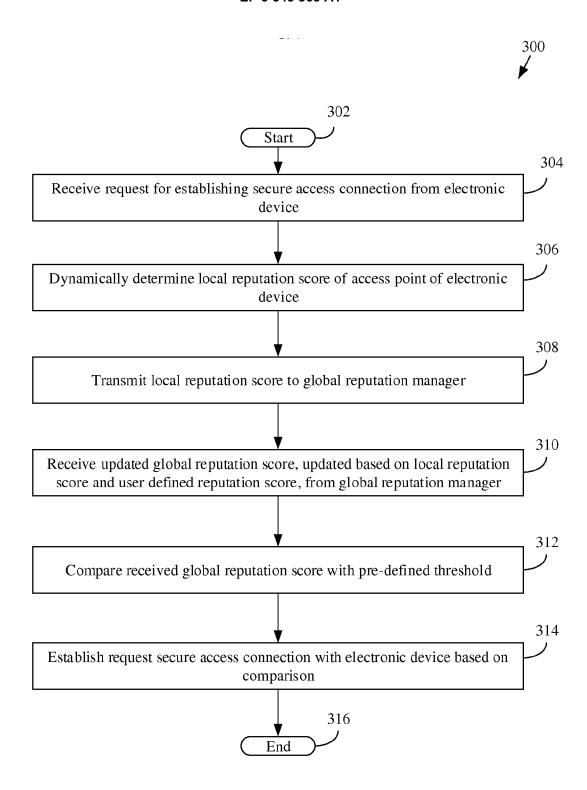
FIG. 3: Method 300 for establishing a secure access connection with electronic devices
