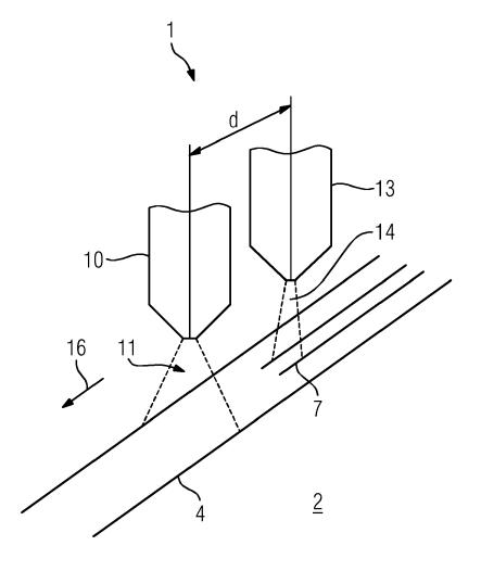
**[0001]** The invention relates to a cladding process wherein two welding heads are used at the same time.
