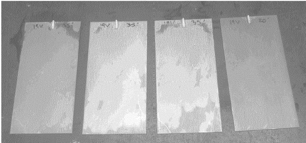
Reverse side salt fog results after 2 weeks
