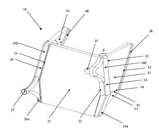
[0001] The present invention refers to a heat exchanger for vehicles which can be used for cooling a thermal engine of a vehicle.
