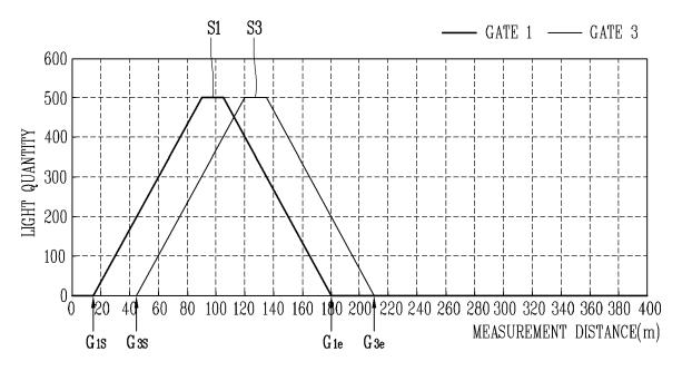
$S_{min} = T_{d} C/2$   $S1 = S_{min} + min(T_p, T_s) C/2$   $S2 = S_{min} + max(T_p, T_s) C/2$  $S_{max} = (T_p + T_d + T_s) C/2$
