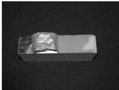
Specimen After Testing Where Adhesion to Foam is Better Than Adhesion to Foil
