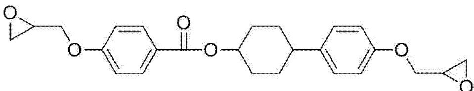
**[0087]** Subsequently, 50 g of Epoxy resin 1 and 9.4 g of 4,4'-diaminodiphenylsulfone as a curing agent were placed in a stainless steel dish, and heated on a hot plate to 180 °C. After the resin in the dish was melted, it was heated at 180 °C for 1 hour. After cooling to room temperature (25 °C), the resin was taken out from the dish and heated in an oven at 230 °C for 1 hour to complete the curing, thereby obtaining an epoxy resin cured product.
