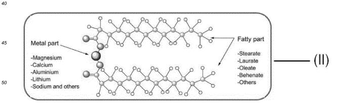
**[0030]** In one of the feature of the present invention, the metal stearate is selected from divalent metal stearate having formula  $C_{36}H_{70}MO_4$ , monovalent metal stearate having formula  $C_{18}H_{35}MO_2$ , and trivalent metal stearate having formula  $C_{54}H_{105}MO_6$ , wherein M is a metal and selected from magnesium, calcium, aluminium, lithium, and sodium.
