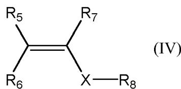
55 Wherein R<sub>5</sub> to R<sub>7</sub> are independently selected from hydrogen, methyl, phenyl or hydroxyalkyl groups containing 1 to 6 carbon atoms, and can be part of a cyclic structure, X is an optionally present spacer group which is selected from -CH<sub>2</sub>-, -COO-, -CONH- or -CONR<sub>8</sub>-, and R<sub>8</sub> is selected from linear or branched, saturated alkyl radicals having 1 to 22 carbon atoms or unsaturated, preferably aromatic, radicals having from 6 to 22 carbon atoms.
