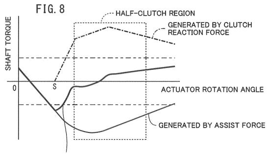
GENERATED BY ASSIST FORCE AND CLUTCH REACTION FORCE
