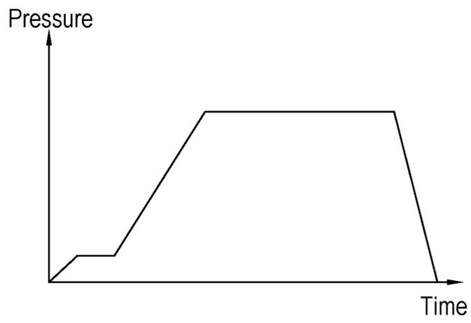
Figure 5 High pressure casting cycle
