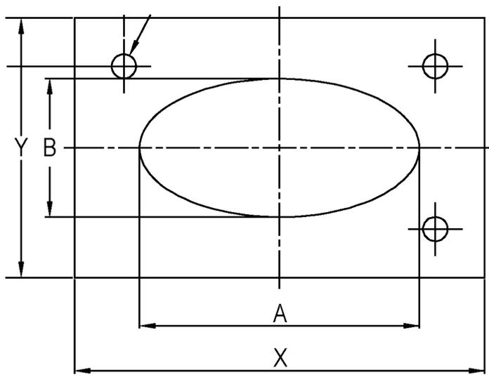
Figure 1 - Active face of a single cavity mould
