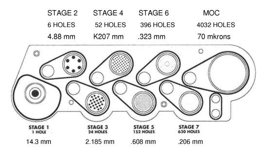
Fig. 1: Schematic drawing of different stages of the NGI (MOC - Micro-Orifice Collector) for Aviptadil
