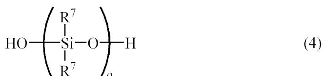
40 wherein R<sup>7</sup> each is identical to R<sup>1</sup>, and q represents a number that satisfies 1 ≤ q ≤ 1,000; (C-3) a silicone resin that contains either SiO<sub>4/2</sub> unit or R<sup>8</sup>SiO<sub>3/2</sub> unit (R<sup>8</sup> is identical to R<sup>1</sup>) as a constitutive unit, and has at least one Si-OH group in a molecule; and (C-4) a silica having a Si-OH group on a surface.
