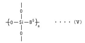
where B<sup>5</sup> represents a single bond or a hydrocarbon group with a carbon number of 1 to 20, a represents an integer of 1 to 10, and a plurality of B<sup>5</sup>, if present, are each independent. As a result of using such a rubber composition in a tire, the low rolling resistance, wet performance, and wear resistance performance of the tire can be highly balanced.
