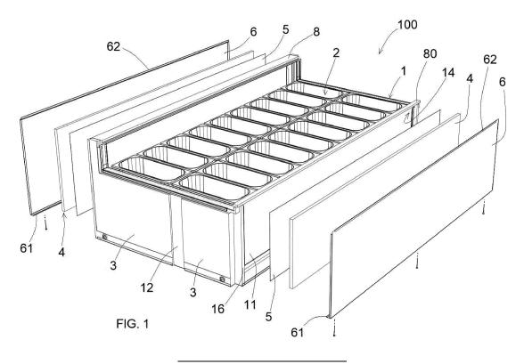
[0001] The present invention relates to a refrigerated display counter with an improved insulation system.
