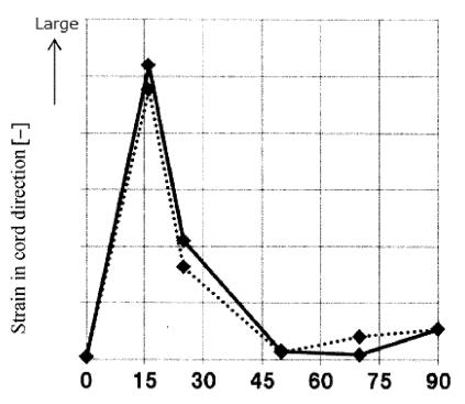
Angle of belt cords of auxiliary belt layer with respect to tire circumferential direction[ $^{\circ}$ ]
