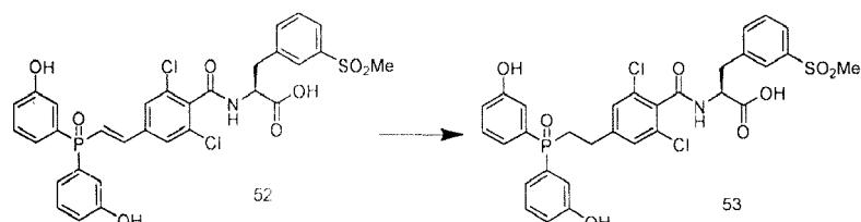
[0302] 12 mg of Compound 52 was dissolved in 0.5 ml of MeOH, 1 mg of 10% palladium carbon was added, and H<sub>2</sub> was added thereto, reacted for 3 hours, filtered, and the product was obtained after purification. LCMS ESI (+) m/z: 677.5 (M+1).
