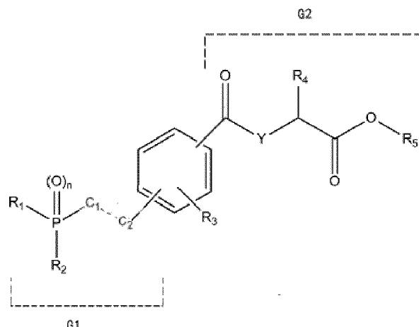
wherein X-Z is replaced by C<sub>1</sub>···C<sub>2</sub> and the carbon bond between C<sub>1</sub> and C<sub>2</sub> is CH<sub>2</sub>-CH<sub>2</sub>, CH=CH or C≡C.
