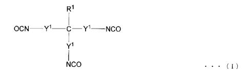
[In Formula (I), a plurality of Y¹'s each independently represent a single bond or a divalent hydrocarbon group having 1 to 20 carbon atoms which may have an ester structure and/or an ether structure, a plurality of Y¹'s may be the same as or different from one another, and R¹ represents a hydrogen atom or a monovalent hydrocarbon group having 1 to 12 carbon atoms.]
