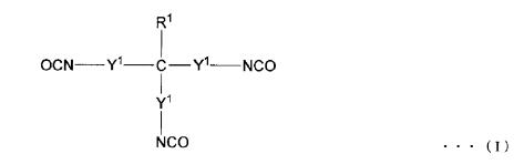
[In Formula (I), a plurality of  $Y^1$ 's each independently represent a single bond or a divalent hydrocarbon group having 1 to 20 carbon atoms which may have an ester structure and/or an ether structure, a plurality of  $Y^1$ 's may be the same as or different from one another, and  $R^1$  represents a hydrogen atom or a monovalent hydrocarbon group having 1 to 12 carbon atoms.]
