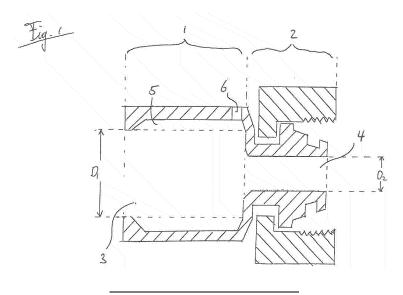
**[0001]** The invention relates to a device for connecting a tubular element, such as a hose or pipe, to another part of a hydraulic or pneumatic system, which device comprises a body having a connection end and a tubular element insertion end, having a cylindrical channel extending from the connection end to the tubular element insertion end, where the connection end serves the purpose of connecting to another part of the hydraulic or pneumatic averter, and wherein the cylindrical channel comp
