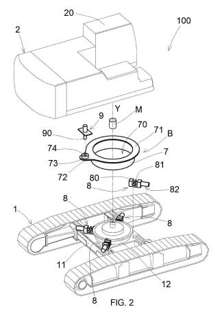
**[0001]** The present invention relates to a drilling machine with telescopic Kelly bar, which is used to drill holes in the ground and is provided with a blocking system suitable for blocking a rotation of an upper unit (tower) relative to a lower unit (undercarriage).
