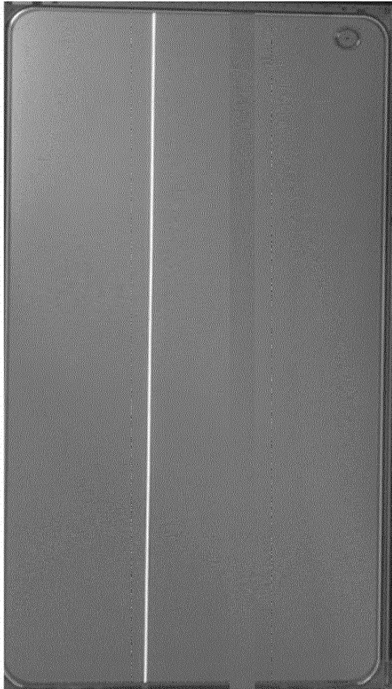
HCD Hole Crack
